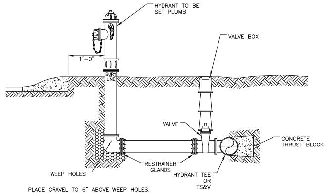
PLACE GRAVEL TO 6" ABOVE WEEP HOLES, 18" BELOW WEEP HOLES AND 18" TOWARDS THE MAIN. ALSO 16" LATERALLY ON EACH SIDE.
